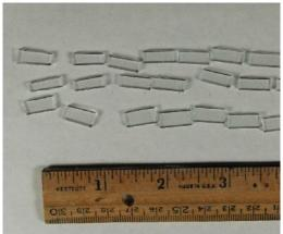
Step 1: Cut strips of glass according to the sizing chart, then cut the strips into rectangles. The length of the pieces will determine your bead size.
