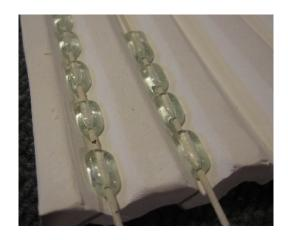
Step 7: After fusing and beads are cool, twist beads off mandrels. Take care to avoid any sharp edges.
