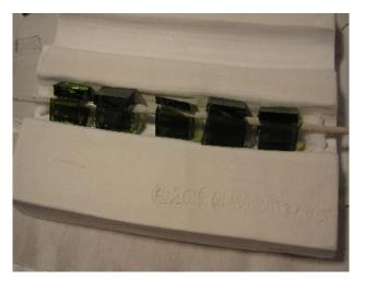
Step 3: Add a second piece of smaller glass to each bead. The small pieces should meet at an angle over the mandrel.
