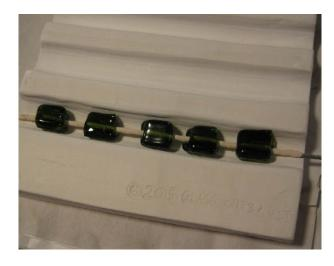
Step 4: Fuse using the firing schedule of page 3. Remove beads from Mandrel after cooling.
