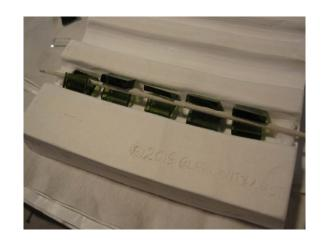
Step 2: Add a prepared mandrel to the glass, brace it with a bit of fiber paper on each end if necessary. Add one smaller piece of glass to each bead on top of the mandrel.
